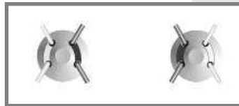
Position 1 (LOAD) Position 2 (INJECT) Flow path of "MX" Nano-Scale Sample Injektor
